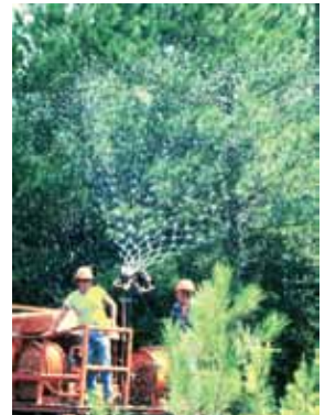
Radiarc® Sprayer produces uniform large droplets.
