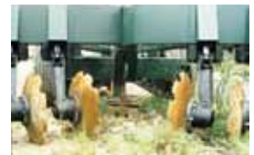
Combination plow with a ripper shank in the center, a wing plow behind, and four disk harrows.
