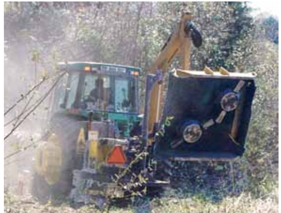
Wetblade system with two cutting heads.
