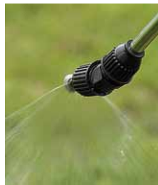
Flooding nozzle spray pattern.
