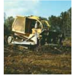
Brush rake attachment for a bulldozer.
