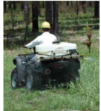
ATV mounted sprayer with a boom.
