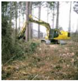
Boom-mounted mulcher head.
