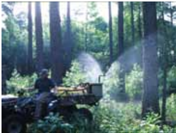
RTV mounted sprayer with Boom-Buster nozzles.
