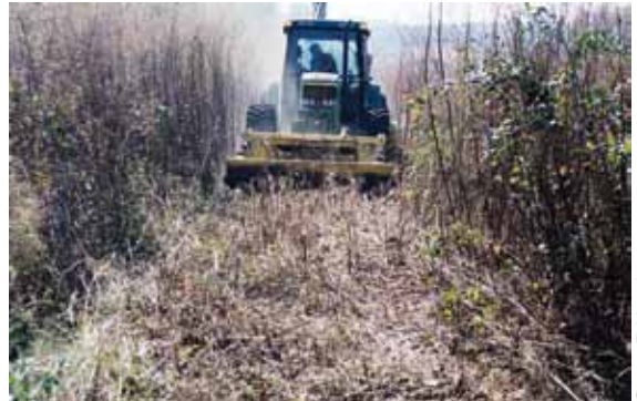
Wetblade brush mower applies herbicide while cutting.
