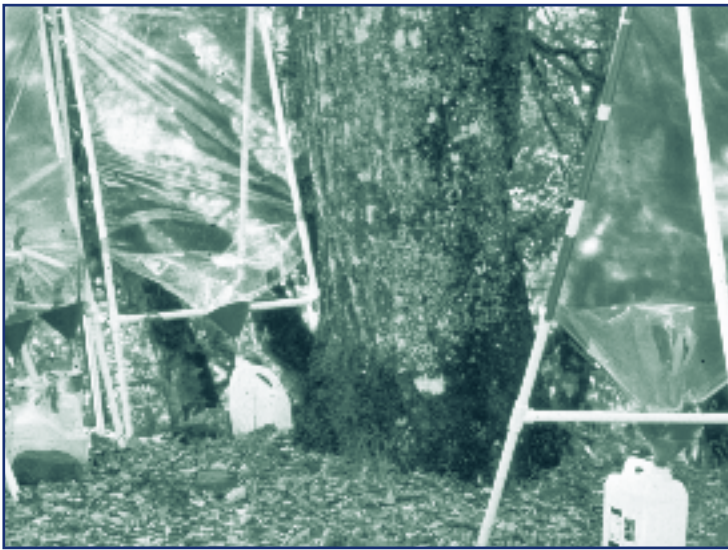
Figure 7. Rainwater traps made out of a vinyl sheet were stretched over a frame and folded over to make a funnel. A 1-gallon jar placed at the end of the funnel collected the rainwater.
